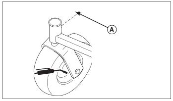
Figure 18. Front Caster & Wheel A. 1/4-28 Bolt
